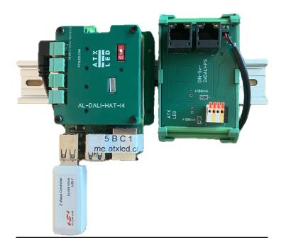
Power source Input Voltage Data (RJ45) Data (KF141) Internal DALI bus supply Raspberry Pi 5v 10w supply Mounting RJ 45 female connector (2) 44-56v DALI bus 2 independent busses see chart DALI bus 2 Yellow / White pairs 2x 80 or 240 mA jumper selectable Provided – specify Mini USB or USB-C DIN Rail
